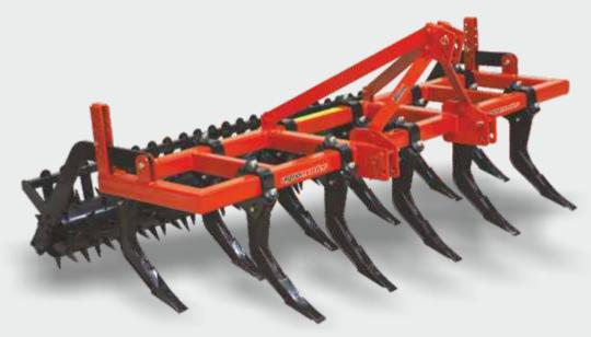
The primary soil tillage machine is mounted from tractor's hydraulic lifting unit and universal three point linkage system. Therefore transportation to the field can be easily done.
