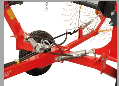
With the adjustable rake wheel down-pressure spring. You can match the rake to your crop conditions. Use less down-pressure for light hay or more down-pressure for heavier hay. By minimizing down pressure, you extend the life of your rake tines and decrease the amount of debris collected in your windrow.
