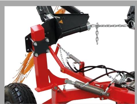
An hydraulically controlled mechanism converts the machine from transport to work position in only a few seconds. The working width and the angle of the finger wheels are easily adjustable to requirements based on the type and conditions of the harvest.
