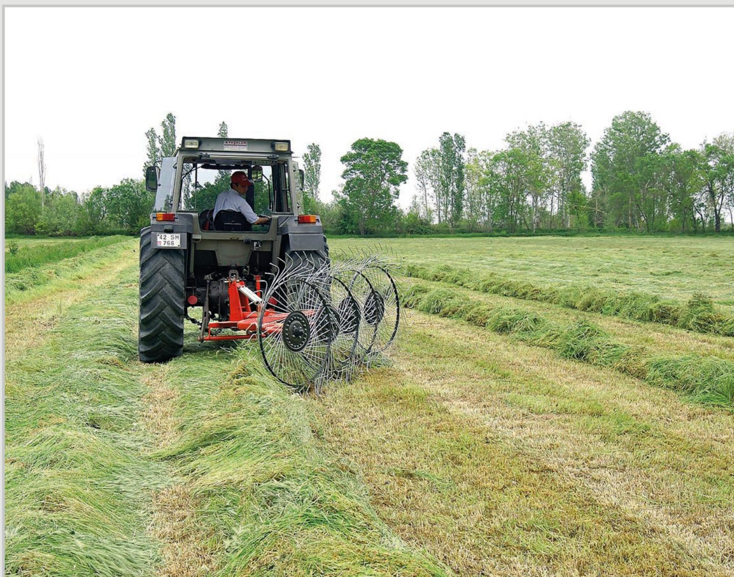
Finger wheel rakes is designed to offer a gentle, crop-driven solution for your grass hay raking needs. This wheel rakes is designed with care and built with quality materials by skilled workers. You get full, nutrient-rich hay that's ready for baling. Available in 8,10 and 12 wheel models
